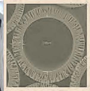
MediSulfone\* UF hollow fiber section. SEM image at 400x
