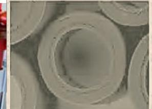
Versatle"-PES hollow fiber section. SEM Image at 300x.
